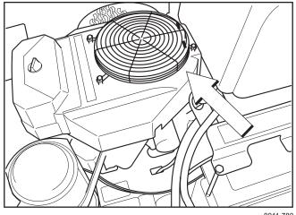
Check and clean the cooling air intake
